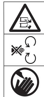
Injury hazard due to rotating blades or other moving parts. Keep hands and feet out of the openings when the machine is running.
